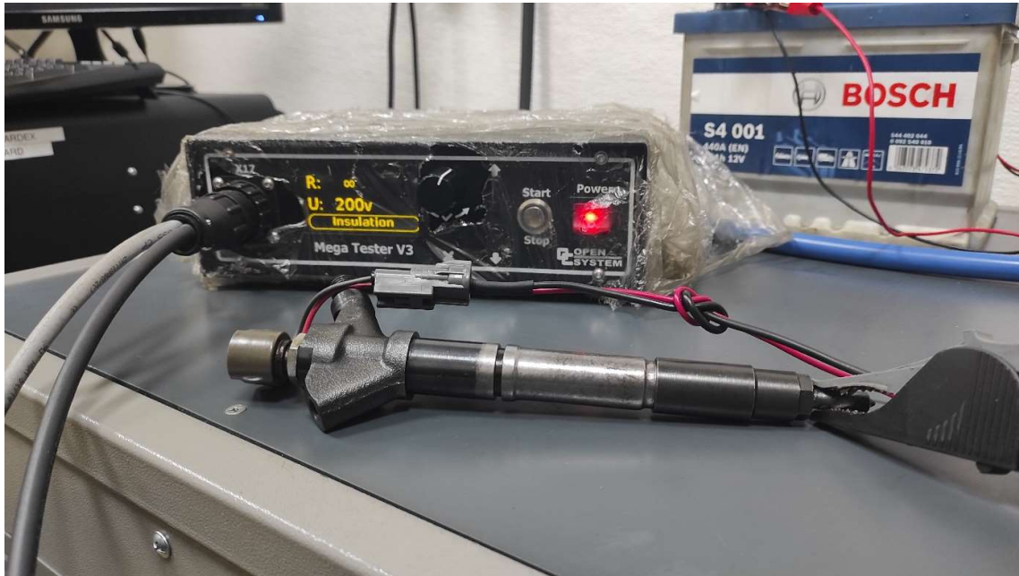
5. Electrical measurements of Denso G2P injector on Mega Tester V3 probe Source: own study
