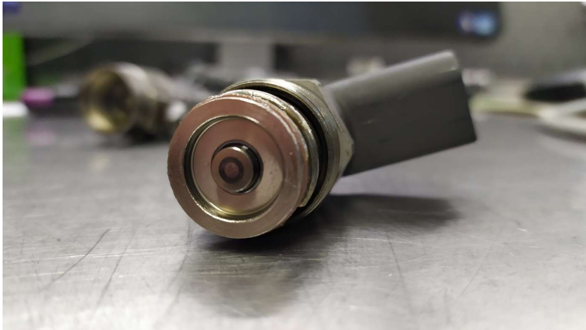
8. Disassembled injector actuator 2.3 PCR from Siemens VDO Continental
