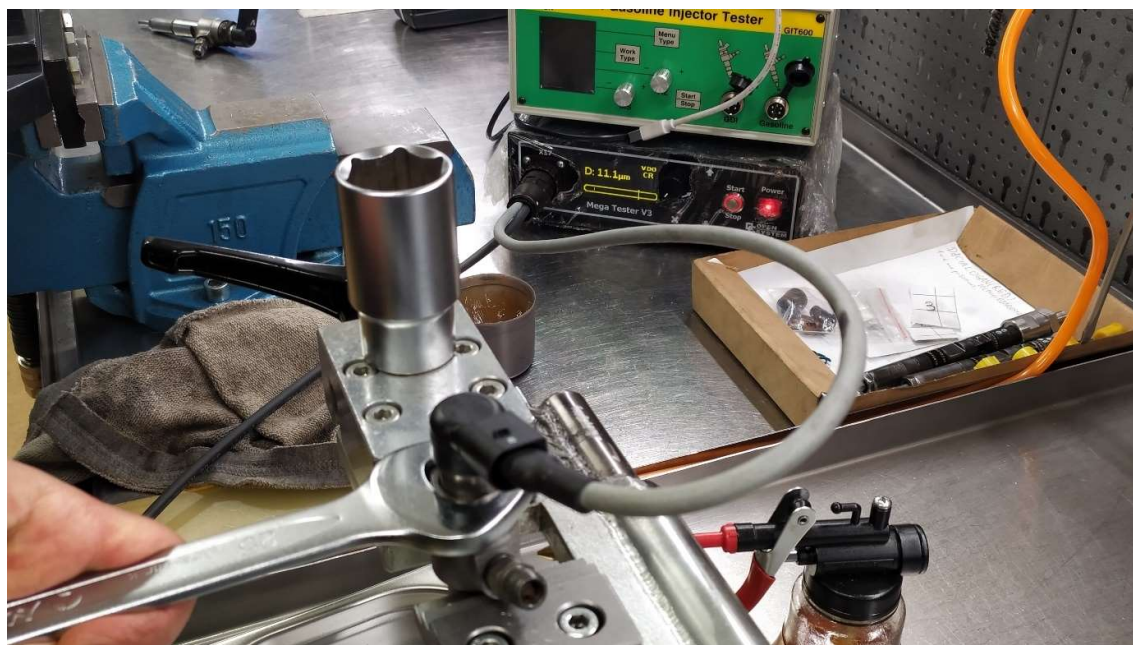
7. Adjustment of the air gap (GAP) in Siemens VDO Continental injectors
