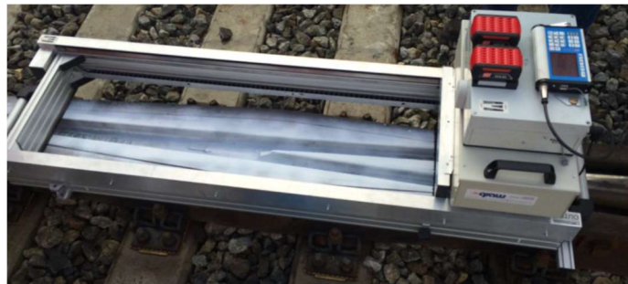
4. 3D Scorpion scanner - intersection in a PPP turnout
