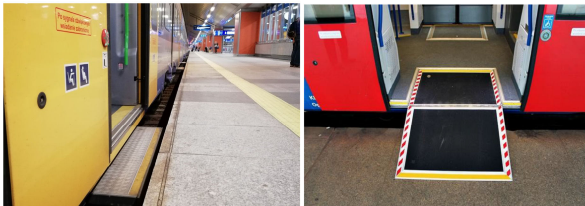
5. An extendable step covering the gap (a) and a folding ramp to the wagon (b)
