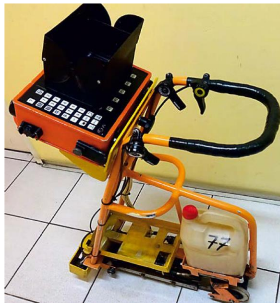
9. RDM-12 trolley for testing railway rails [6]
