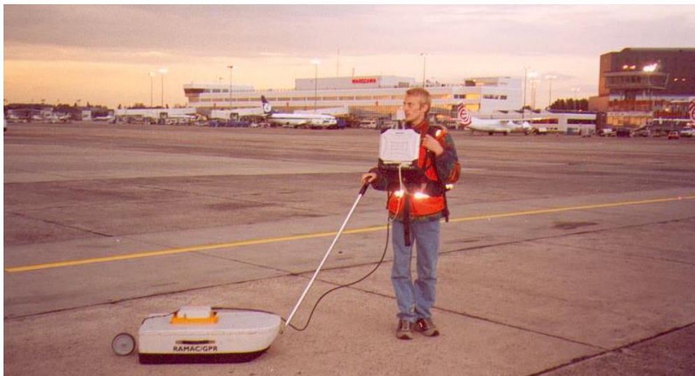
1. RAMAC/GPR equipment with 250 MHz shielded antennas
