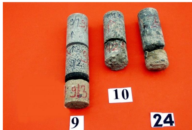
2. Examples of cores from drilling in pavements: 9 - core from the new pavement, 10, 24 cores from old pavement
