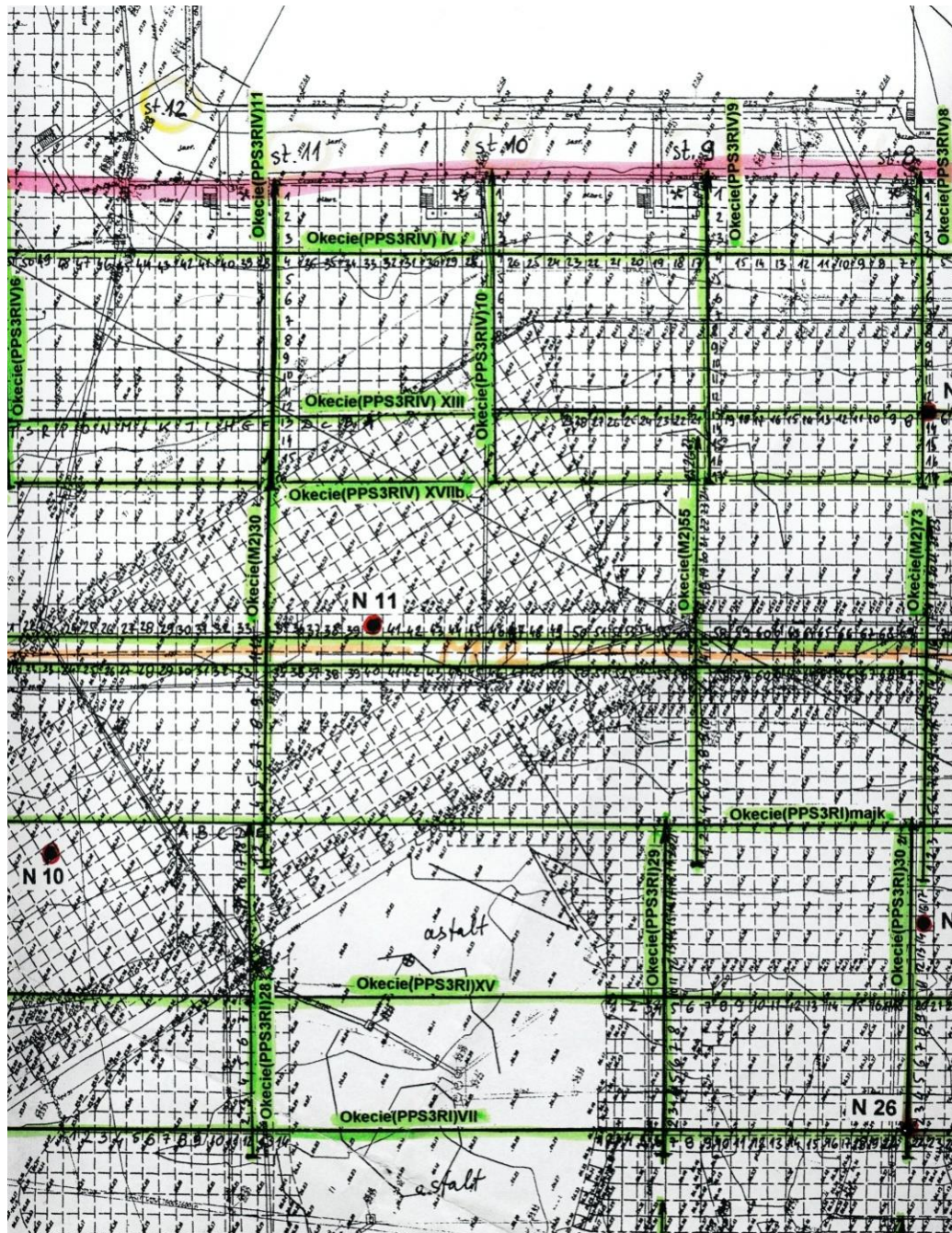
4. Location of selected GPR cross-section lines (green line) and selected pavement drillings
