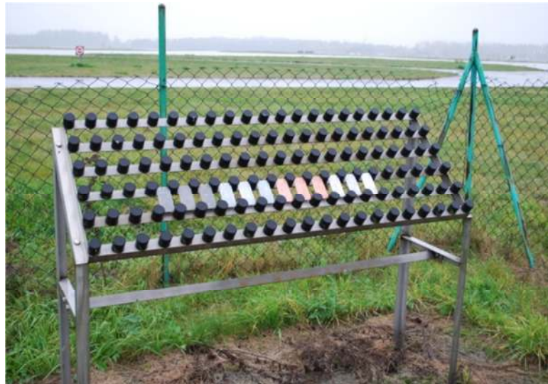
2. An example of a corrosion station located at one of the airport facilities
