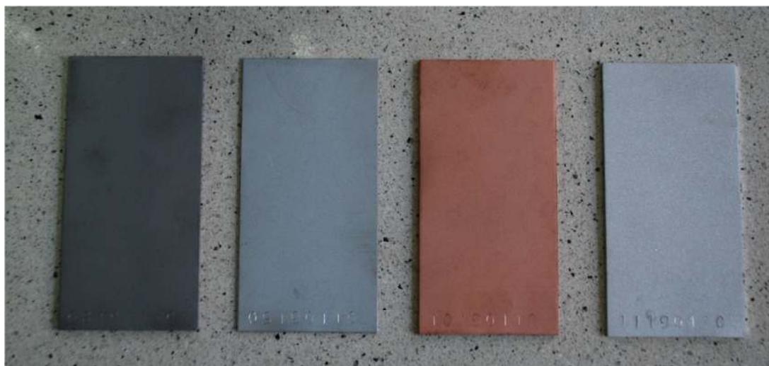
4. Reference samples after air sandblasting and their labeling
