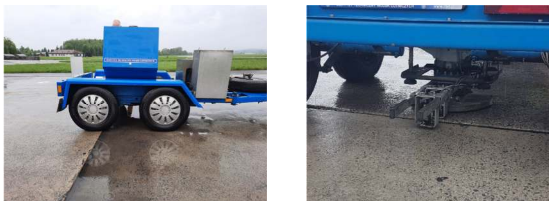
11. HWD impact deflector during measurements of elastic deflections
