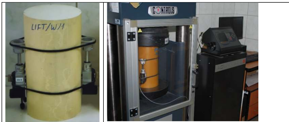
4. Testing the modulus of elasticity of a sample of material for geotechnical injection, a) a sample of Cover Geolift 2K material prepared for testing b) a view of a sample of Cover Geopur 2K in a testing machine
