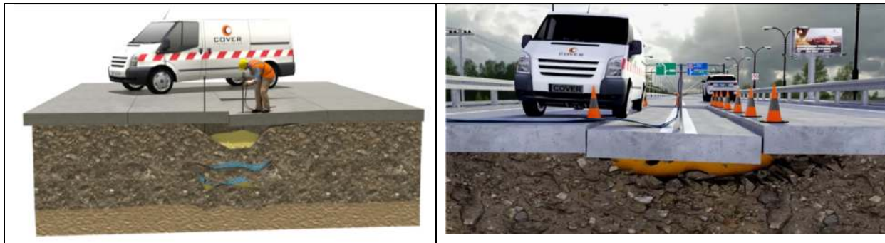
2. The use of geotechnical injection to lift the slab in the concrete pavement
