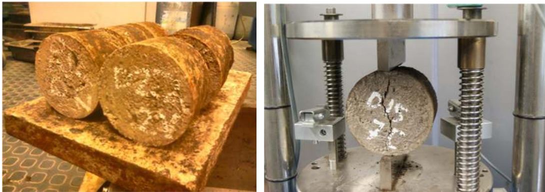
2. Indirect tensile strength ITS specimens and test scheme
