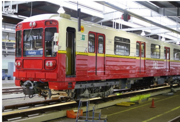
1. 81 series 81572P and 81-573P vehicle. Vehicles with DC drive units (24 x 110 kW) on each axle. The car body is a welded steel structure. Vehicle weight 200 tons
