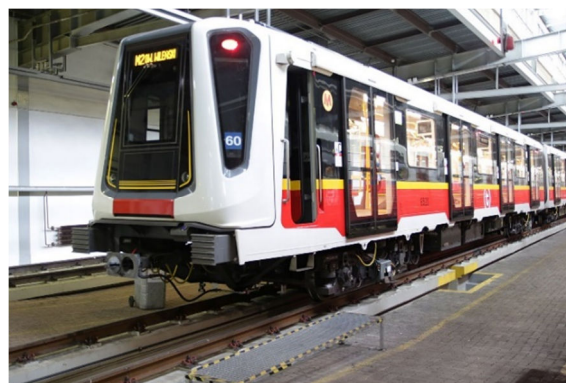
3. Inspiro type vehicle. Vehicles with AC units (16 x 160 kW). The car body is an aluminum construction. Vehicle weight 165 tons
