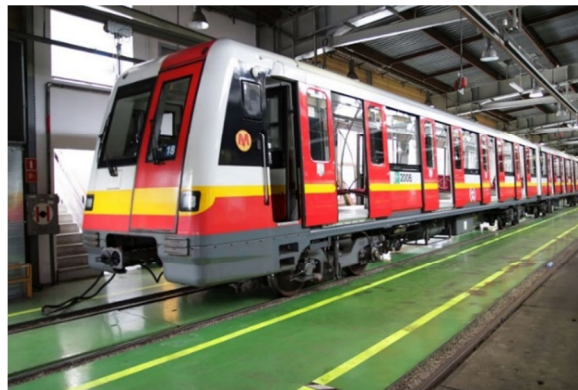
2. Metropolis type vehicle. Vehicles with AC units (16 x 180 kW). The car body is an aluminum construction. Vehicle weight 186 tons
