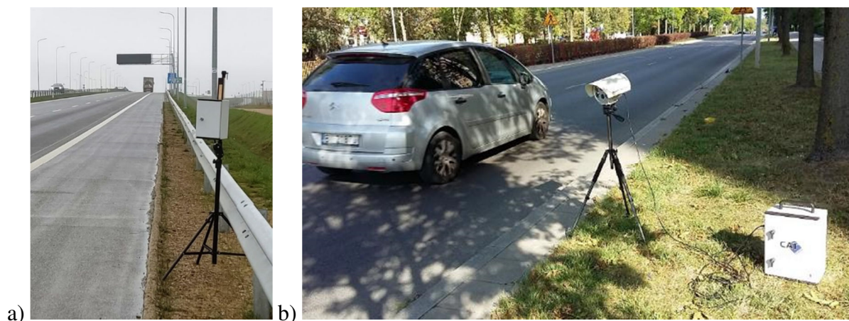
6. Apparatus for measuring the speed of vehicles: a) instantaneous - Sierzega SR4, b) segmental - ANPR camera (one of two on the section)
