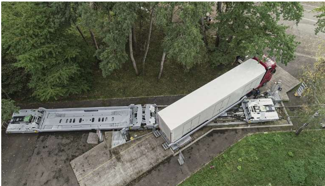
3. Semi-trailer on the loading front of the Modalohr subsystem (Source:[3])
