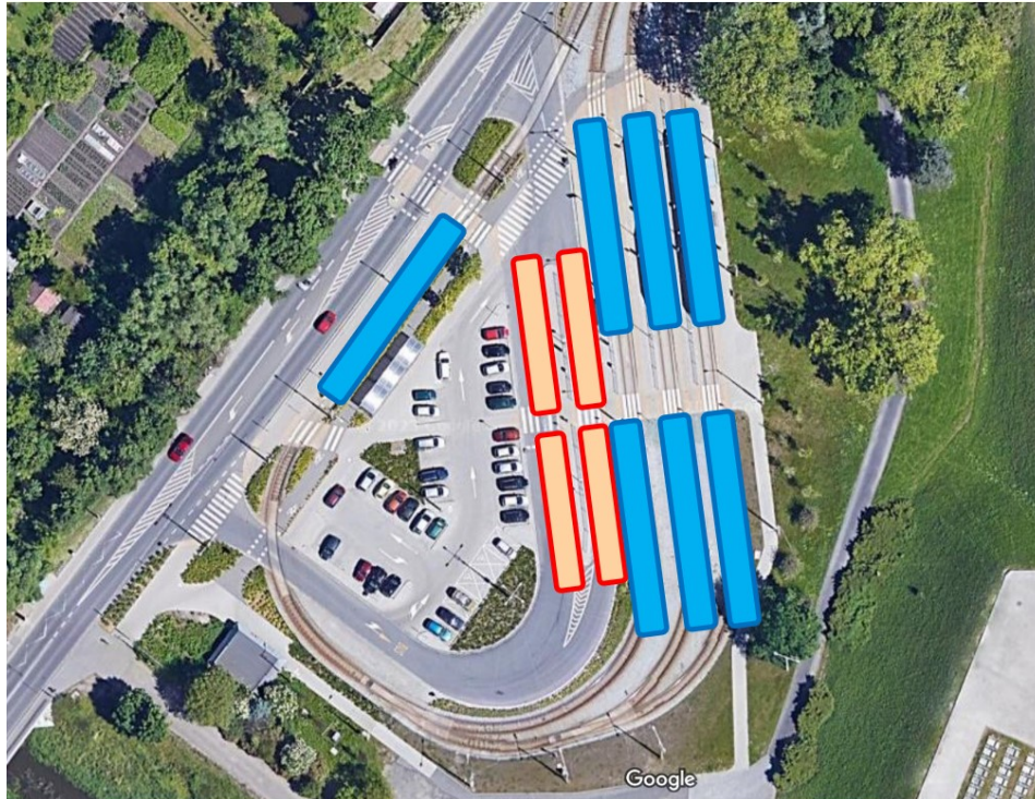
6. Resistance Loop, number of vehicles including the vehicle on the platform for getting off and vehicles waiting to enter the platforms, 11 in total.
