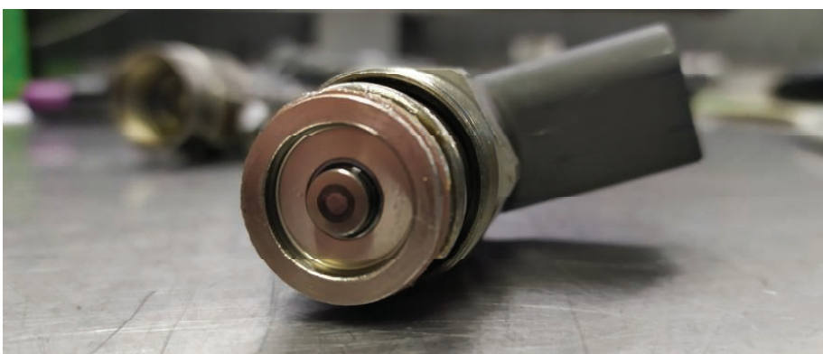
8. Disassembled injector actuator 2.3 PCR from Siemens VDO Continental Source: own study
