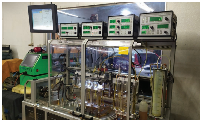
3. Modular test station STPIW-3 (Autoelektronika Kędzia) Source: own study
